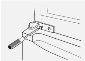
24. plug the pin of the upper hinge in the fixture of the upper appliance door.
