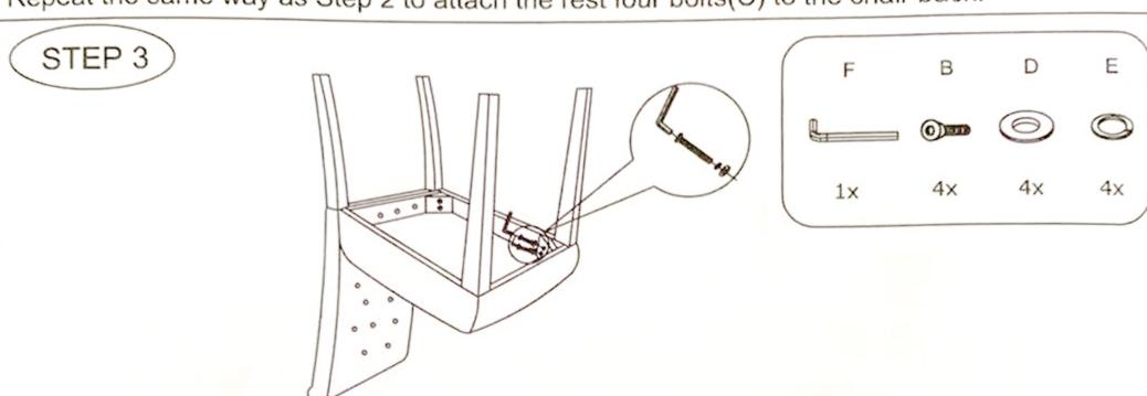
Insert the front legs (3) to the seat frame by using spring washer(E) and flat washer (D), bolt(B), with allen wrench (F).
