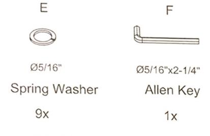
NOTE:Straight Allen Key(F) is for use with a power drill.
