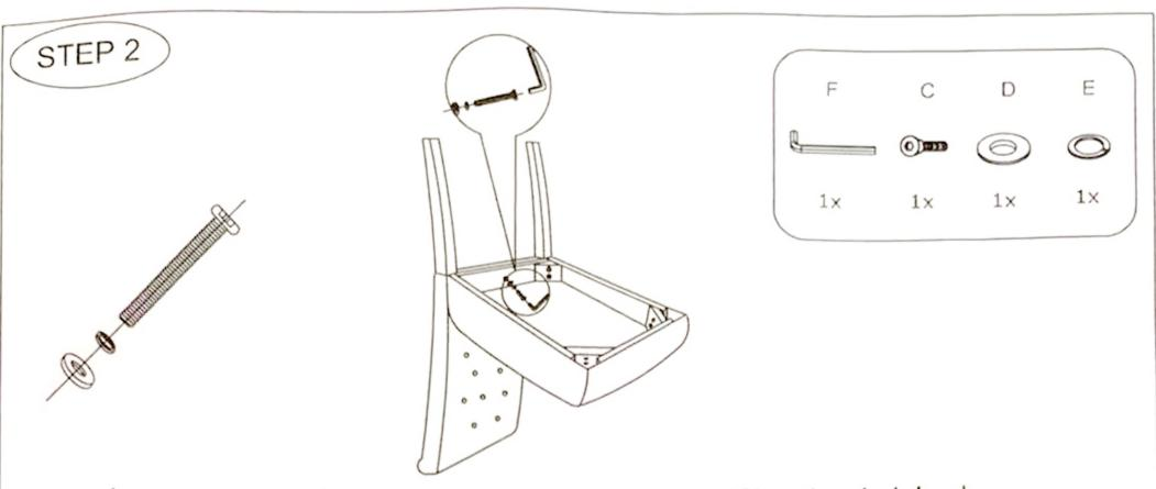
Repeat the same way as Step 2 to attach the rest four bolts(C) to the chair back.
